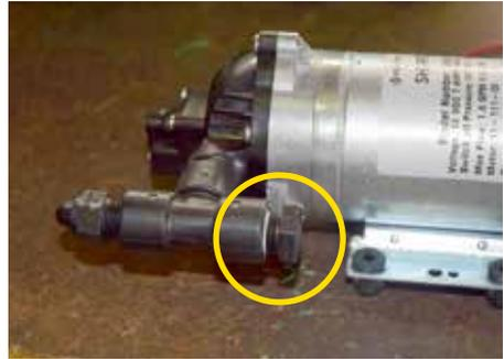
8 Fit GA5077700 hose barb to pump using sealant.
