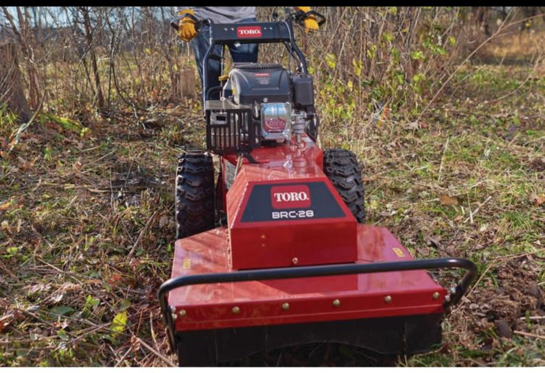
This versatile machine is ideal for the rental and landscape contractor industries, as performance, durability and usability are key elements in its design. The commercial grade, self-propelled brush cutter allows operators to level brush, tall weeds, saplings and heavy vegetation with ease. The Toro hydro drive brush cutter, featuring a pivoting deck, can handle brush up to 1.8 metres tall and saplings up to two 50 mm.
