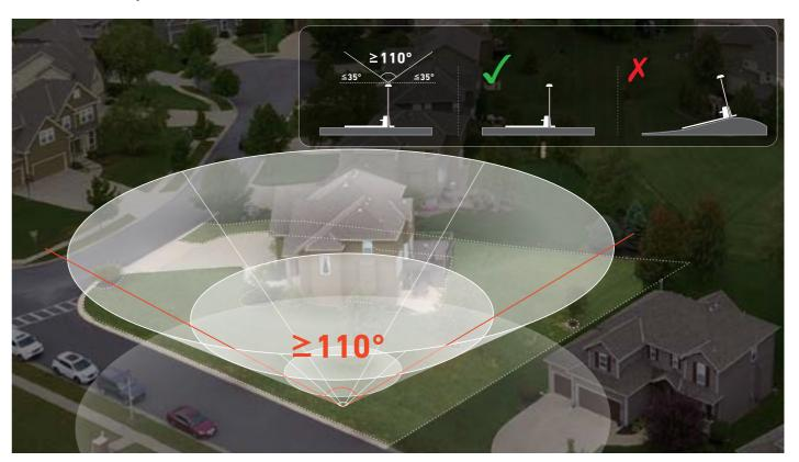
To get better signal, you can purchase the antenna extension kit and install it according to the provided instructions, ensuring an unobstructed sky view of at least  $160^{\circ}$ .
