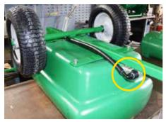
8 Fit GA5077700 hose barb to pump using sealant.
