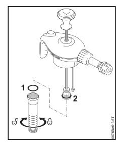
Unscrew the pump barrel and pull it off the piston.
