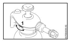
Turn the knurled wheel (1) as far as stop and hold it there until the tank is no longer under pressure.
